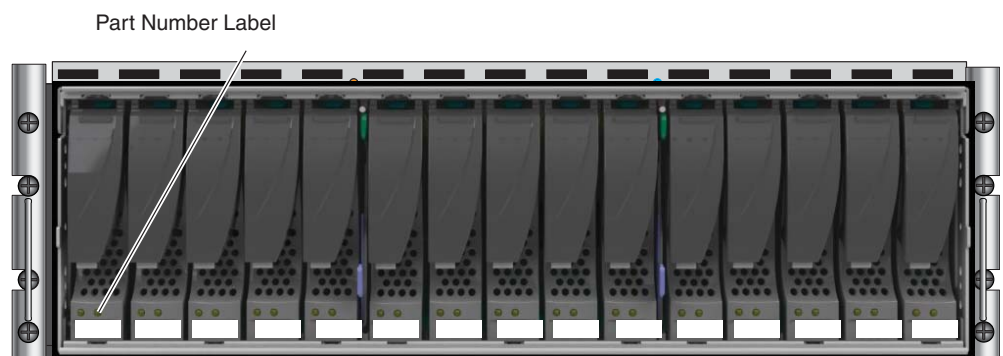
Figure 35 Example of the 3U, 15 (3.5-inch) disk drive DAE (front view)
