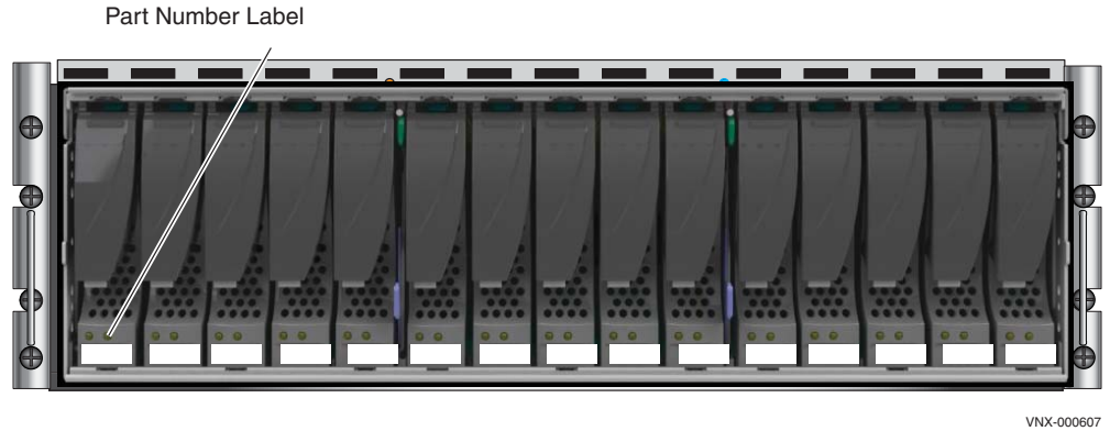
Figure 5 Example of the DPE 3U, 15 (3.5-inch) disk drive (front view)
